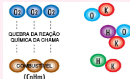
The potassium free radicals react with the O, H e OH, removing them from the flame, producing KO, KH e KOH.
